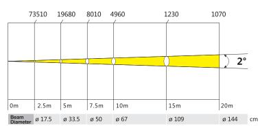
The MINIBEAM 50 features a 50W LED with high intensity and efficiency. It produces very high light output much higher than the 90W beam, through a specific 2° optic system. The PAN/TILT integrates in fast and quiet movement. It offers a full complement of professional characteristics, including a static gobo wheel (17 gobos plus open), a color wheel (14 colors plus open), a 8-facet prism, 0-100% linear LED dimmer, variable speed shutter/strobe.
