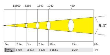
The MINISPOT 50 features a 50W LED with high intensity and efficiency. It produces very high light output similar to a 90W spot, through a specific 9.4° optic system. The PAN/TILT integrates in fast and quiet movement. It offers a full complement of professional characteristics, including a rotating gobo wheel (6 interchangeable gobos plus open), a color wheel (7 colors plus open), a 3-facet prism, motorized linear focus, 0-100% linear LED dimmer, variable speed shutter/strobe.
